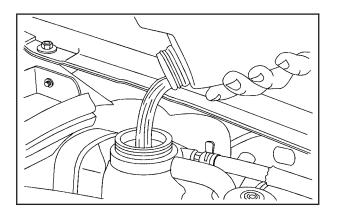
Fill the coolant surge tank with the proper DEX-COOL<sup>®</sup> coolant mixture, to slightly above the FULL COLD/FROID line on the side of the coolant surge tank.
